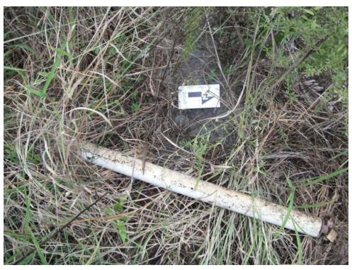
Photograph 8: View of 2-inch diameter monitor well (found to be broken at land surface).
